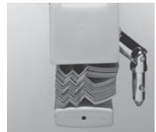
Fig. 11: Optics of the mono-reflective daylight system RETROLux 50 for the interior space. By avoiding otherwise common pendulum reflections of the scattered radiation on the louvers, the RETRO louver is optimized in terms of the photometric and energetic behavior.
